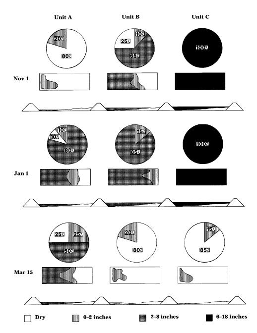
**Fig. 3.** Planned flooding strategies for three moist-soil units during one winter season. The initiation, depth, and duration of flooding are different for each unit. Note that two of the three units were never intentionally flooded to capacity. This does not mean that natural events would not flood the unit to capacity. Flooding strategies should be varied among years to enhance productivity.
